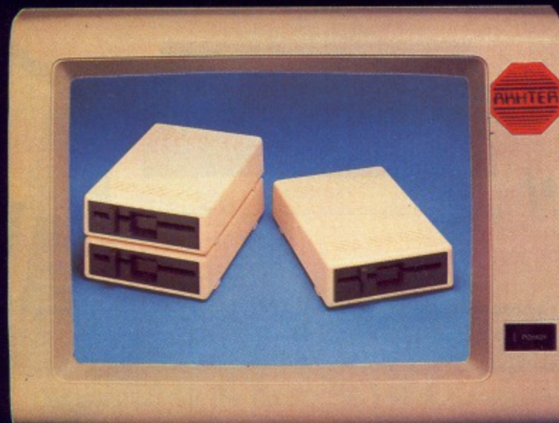
Single 5 1/4" drive, without power supply, in a plastic case. [Code suffix 'A' see opposite page]. Dual 5 1/4" drives, without power supply, in a plastic case. [Code suffix 'C' see opposite page].
